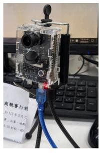
The AMB82 mini development board can be connected to various electronic components such as LEDs, switches, pressure sensors, humidity sensors, and PM2.5 dust sensors. The collected data can be uploaded via WiFi for use by applications, enabling the realization of IoT applications.
